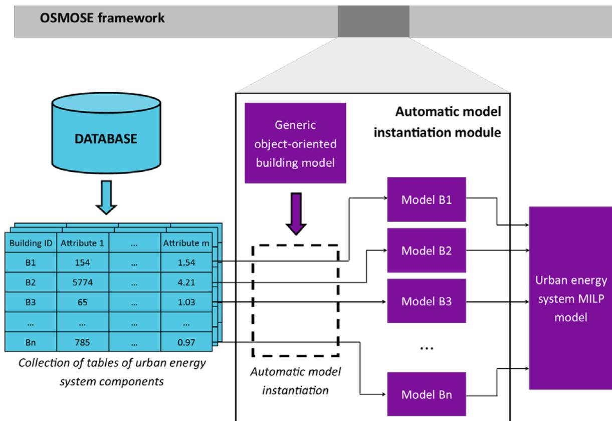
Figure 5 - Automatic urban energy system model instantiation module
