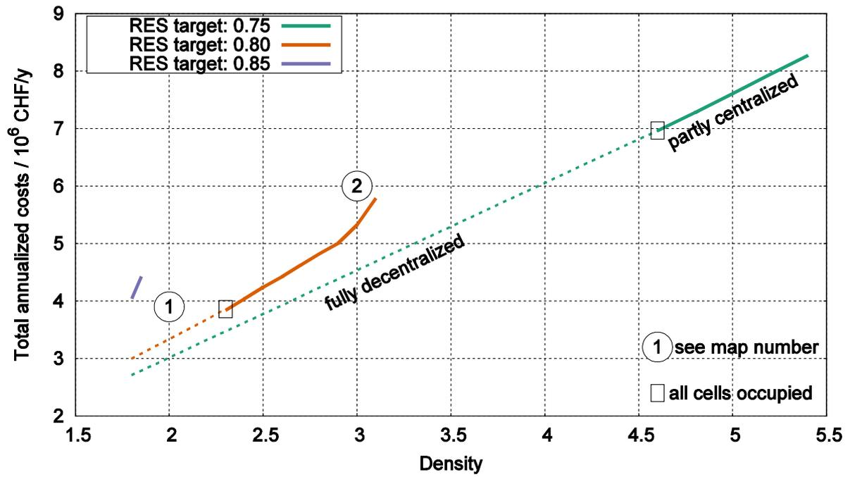
Figure 8 - System costs for different RES targets, over varying density [1]
